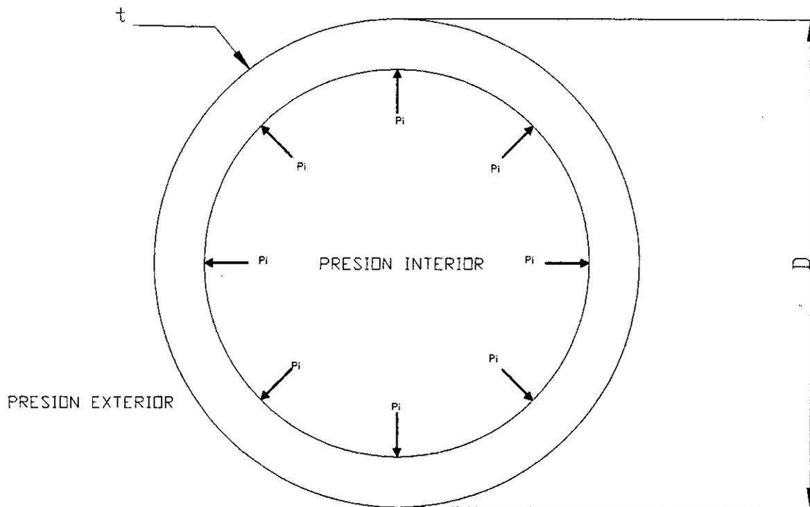
Donde:  $t = \text{espesor}$   $t \geq 1,25 \frac{PxD}{2\sigma_{adm}} + 0,003m \dots \dots \dots (4-8)^{(5)}$
