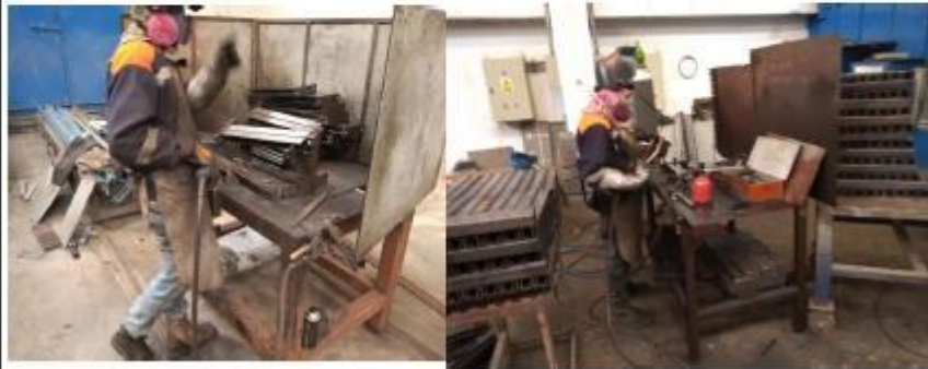
View of ladder trays in the welding process, the trays are being welded with a drawing without FLUOR approval.
