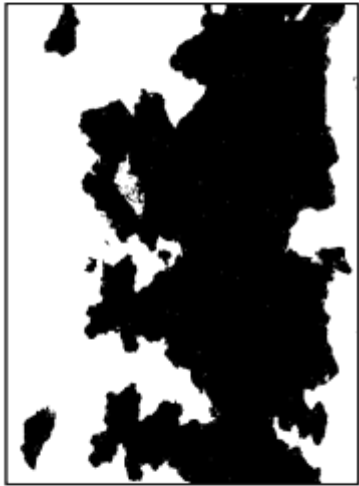
Rust Grade 1-G, 50% Rusted
