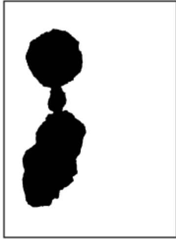
Rust Grade 3-S, 16% Rusted
