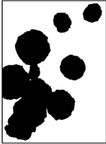
Rust Grade 2-S, 33% Rusted
