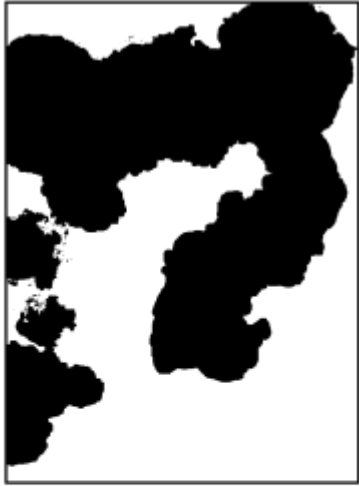
Rust Grade 1-S, 50% Rusted
