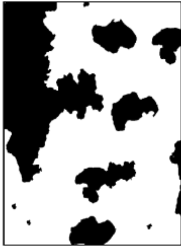
Rust Grade 2-G, 33% Rusted
