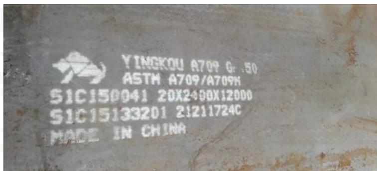
*Figura 22: Plancha de acero al carbono ASTM A709 Gr 50*
