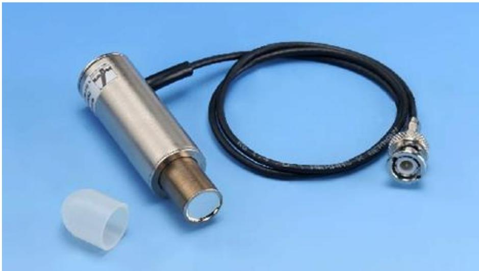
*Figura 22.* El Contador Geiger-Müller. Adaptado de PHYWE Series of Publications, TESS extert, Laboratory Experiments, 2016, Copyrigh 2016 por PHYWE Systeme GmbH & Co.
