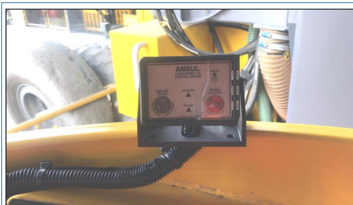
Figura 3-15: Cabletec M, Checkfire sistema Ansul
