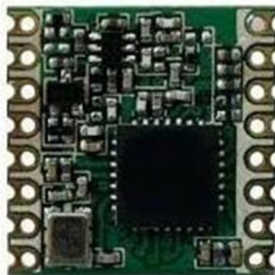
Figura 10. Transceptor LoRa RFM95W de 915 MHz
