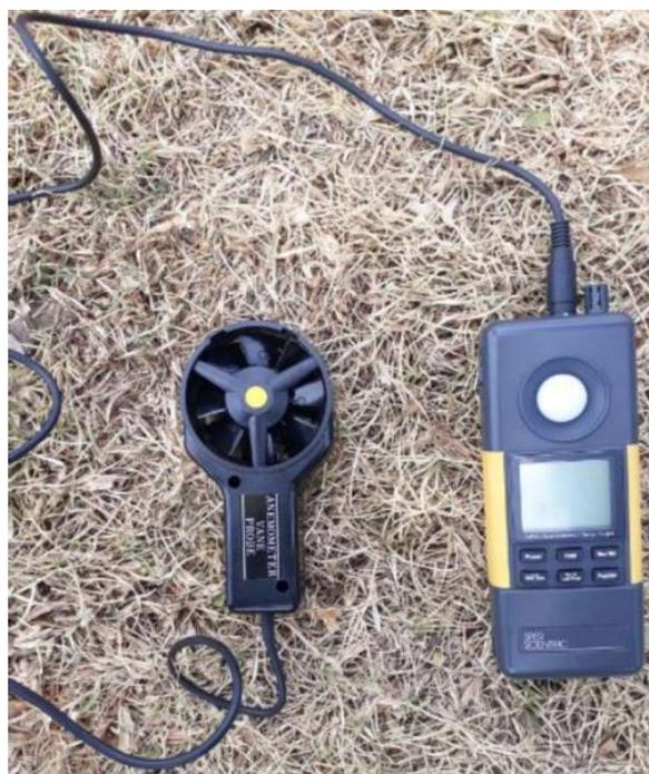
Figura 13. Hybrid-Powered Environmental Quality Meter 850068
