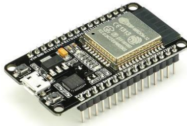
Figura 2. Firmware open source node MCU 32
