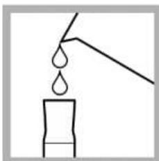
2. Fill a 25-mL graduated mixing cylinder with 20 mL of sample.
