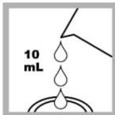
2. **Prepare the sample:** Fill a sample cell with 10 mL of sample.
