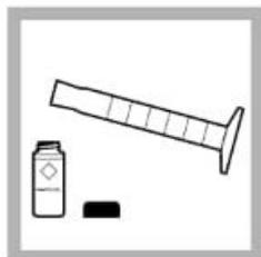
5. **Prepare the blank:** Fill a sample cell to the 10-mL mark with the solution.
