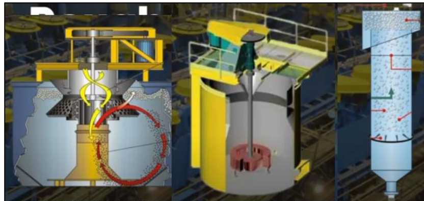
Figura 2.23 Celdas rougher /scavenger/cleaner
